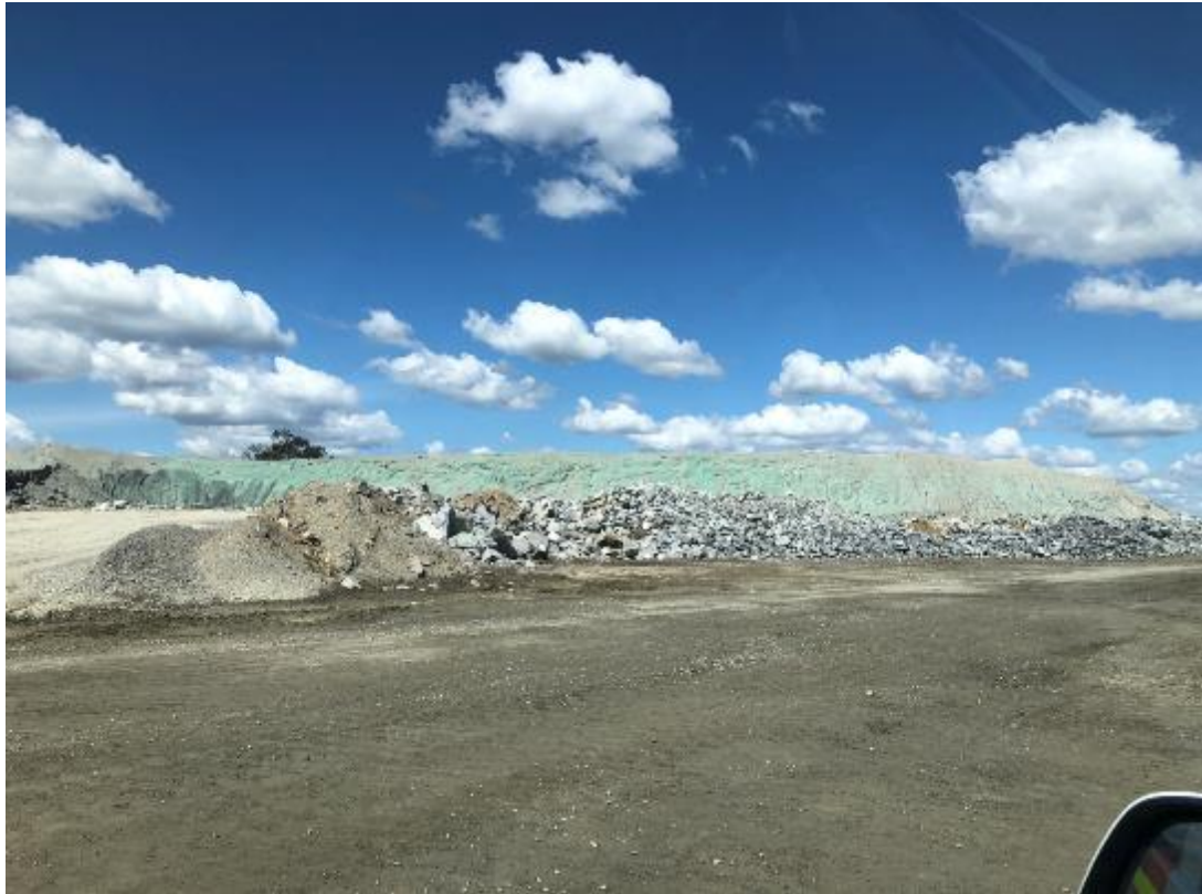
Figure 12: Dust suppression (polymer) applied to product stockpiles
