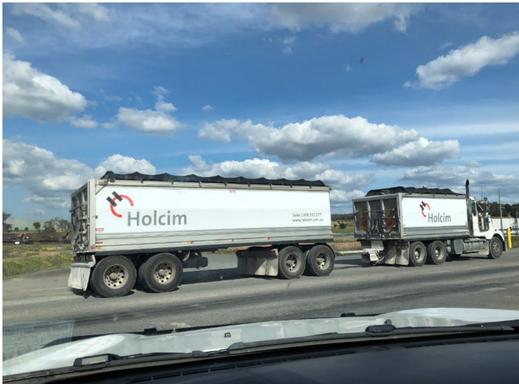
Figure 3: Covered loaded truck leaving site
